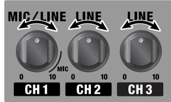
Adjust the volume balance for CH 1 through CH 3 at this time.
