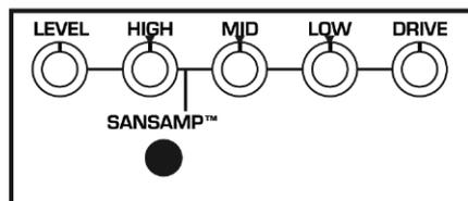
**DRIVE:** Adjusts the overall amount of gain and overdrive, similar to when the output section of a tube amp is being pushed. The first half of the rotation will increase the volume as well as the overdrive.
