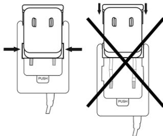
Press the PUSH switch to release the prong assembly. Slide the assembly up (about halfway) to align the side tabs of the prong assembly with the slots of the power supply housing. Then pull up to remove the assembly. Choose the new prong assembly, align the side tabs with the slot of the housing and slide down until it clicks into position.
