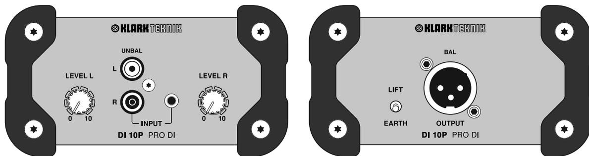
**INPUTS** – Connect your source audio via stereo RCA jacks or a single 1/8" TRS jack. The unused input jack can act as a loop-through output. A mono source can also be connected to one of the RCA jacks, or to the 1/8" input.
